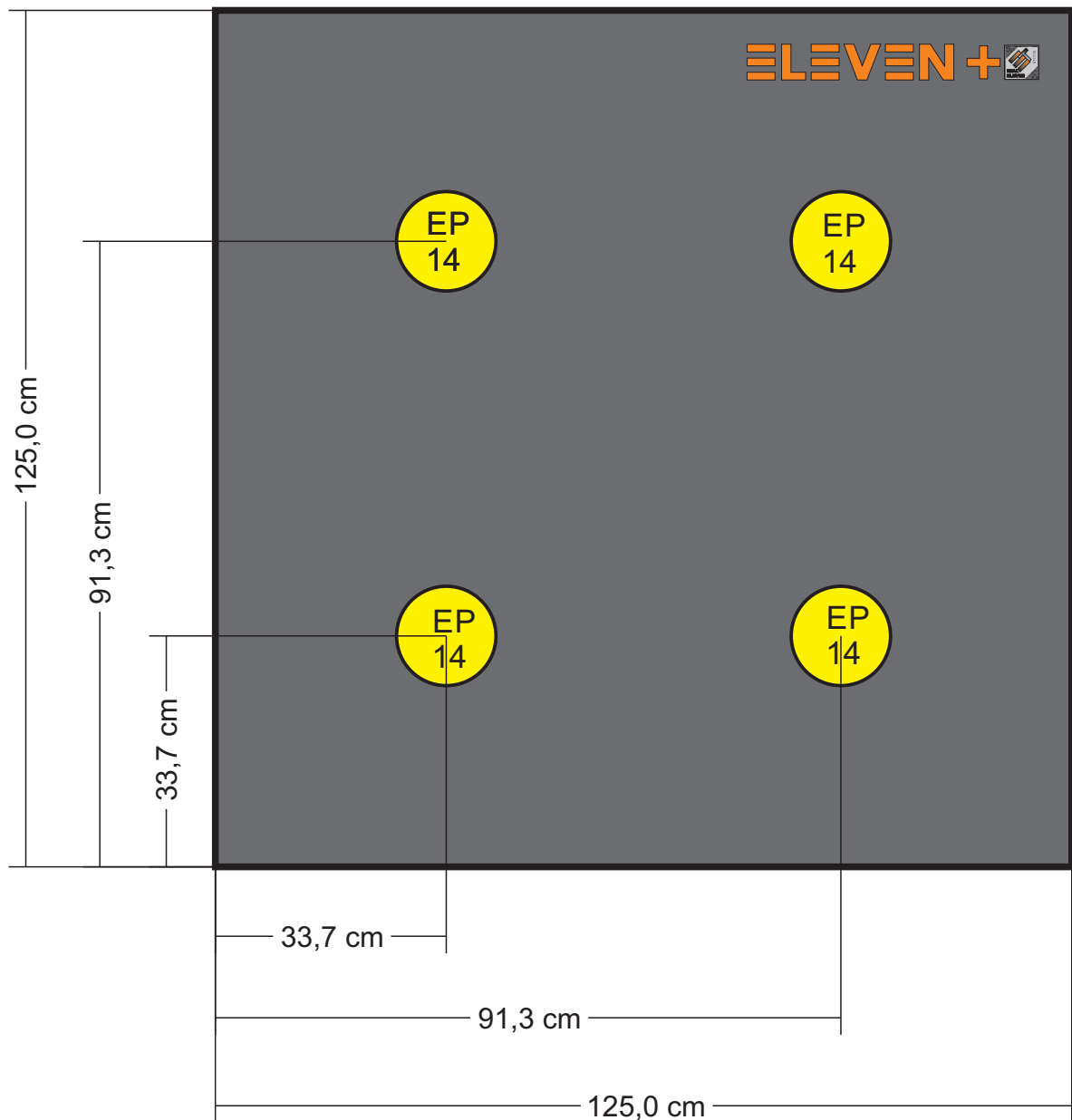
ELEVEN+ Buttruss 125x125 cm with 4 pieces 14,5 cm EP inserts for qualification round of compound divisions
